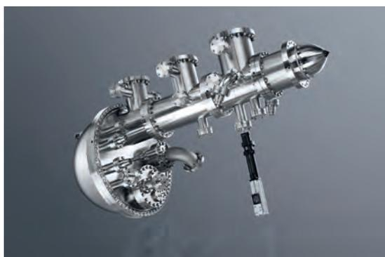
For analysis in pressures up to 25 mbar the lens system is a crucial part of the NAP electron spectrometer design. The first aperture (nozzle) has a diameter of down to 0.3 mm, separating the wide-angle lens from the sample environment. Together with the standard PHOIBOS lens it forms a three stage differential pumping system.
