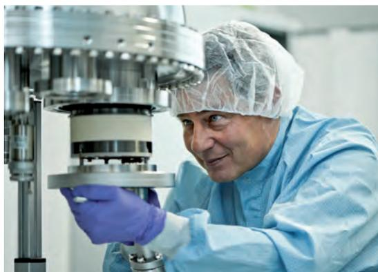
SPECS specialist assembles a high voltage 2D-CCD Detector to a PHOIBOS 150 HV
